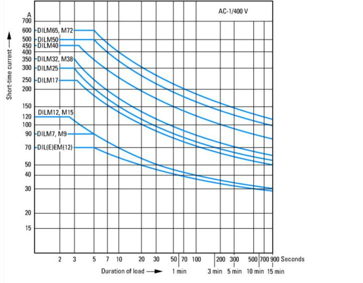
Short-time loading, 3-pole Time interval between two loading cycles: 15 minutes
