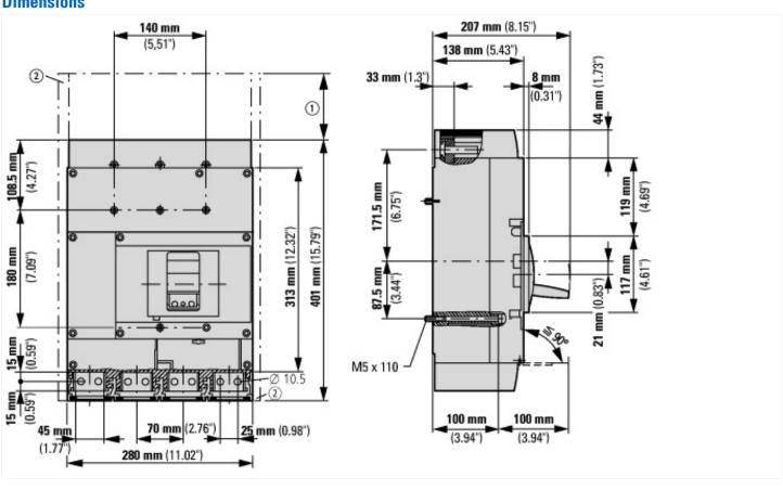
Blow out area, minimum clearance to other parts \( \leq \) 260 mm
