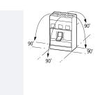
With residual-current release XFI: - NZM1, N1, NZM2, N2: vertical and 90° in all directions 90° in all directions
