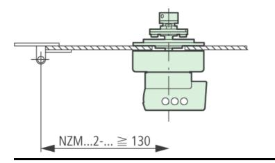
Minimum door coupling rotary handle clearance from door pivot point
