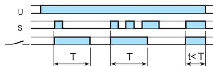
**(DE) Interval with control signal on.**
