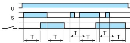
**(CE) On- and off-delay with control signal.**
