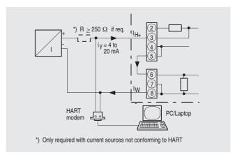
SIPART PS2 electropneumatic positioner, example of connection for communication through HART for 6DR52..
