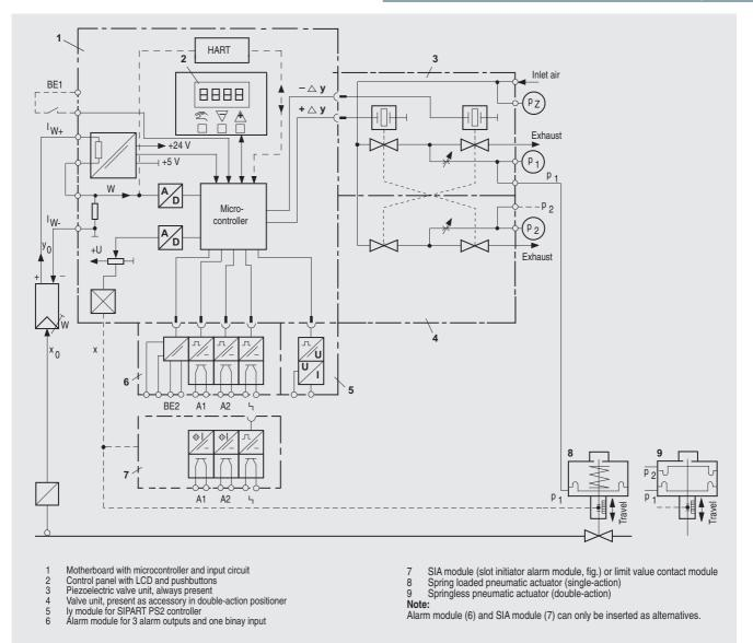
SIPART PS2, electropneumatic positioner, function diagram
